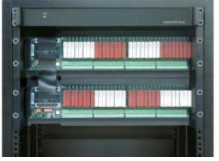
The 64-channel isolated discrete I/O system consists of one DaqScan/2002 plus two DBK210 boards with rack-mount kits
