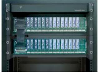
The 24-channel isolated system includes a DaqScan/2005 plus two DBK207/CJC boards. The system is capable of scanning all channels at 5 µsec per channel, and provides 500V isolation for all inputs.
